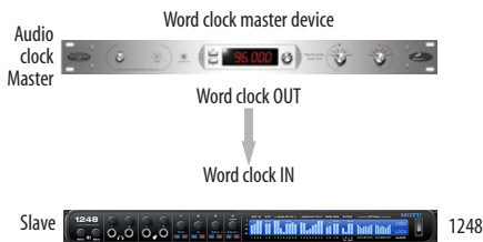
Figure 4-19: Slaving your MOTU device (a 1248 in this example) to word clock. For the 1248 clock source, choose 'Word Clock In'.
