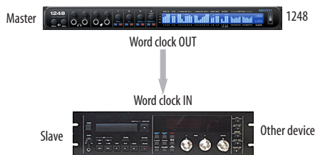
Figure 4-18: Slaving another digital audio device to your MOTU device (a 1248 in this example) via word clock. For the 1248 clock source, choose any source besides word clock, as it is not advisable to chain word clock.
