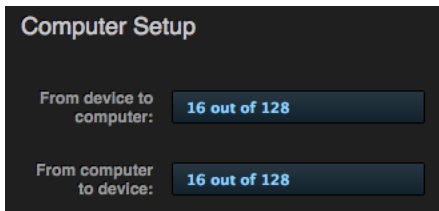
Figure 9-2: The 'From device to computer' setting determines how many channels you see in the Left Input and Right Input menus.
